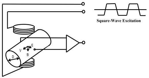
Figure 14.1 Principle of Operation
